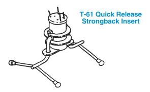
The T-61 Quick Release Strongback Insert is designed to provide access for the strongback hardware and adequate lifting capacity for the assigned project. The insert is furnished as an assembly, complete with locator cap and plastic tipped feet
