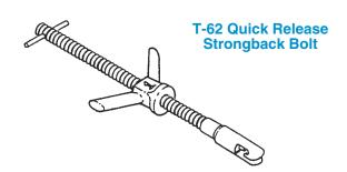
The Dayton Superior T-62 Quick Release Strongback Bolt is a simple coil threaded unit designed to quickly engage and tie strongback beams to a tilt-up concrete panel. The unit requires no tools for installation or removal and works well with steel, aluminum or wood strongbacks.
