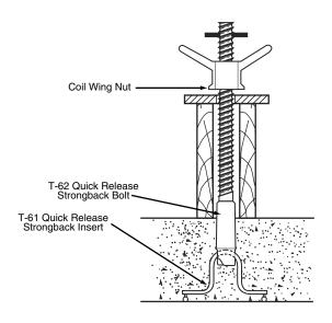
Warning: Strongbacks are intended to stiffen tilt-up panels and are not to be used for attaching the lifting apparatus. Failure to heed this warning may result in a panel failure and/or personal injury.
