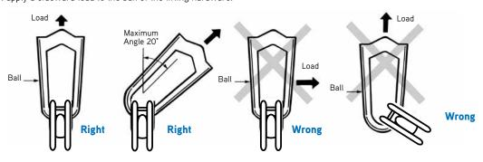
Warning! Do not modify, weld or alter in any way T120 Hardware units. Such actions could lead to premature failure of the hardware.
