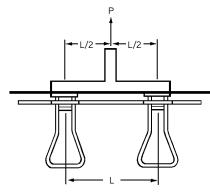
Note: To achieve Safe Working Load, Lifting Plate must be centered on T3 or T11 Insert
