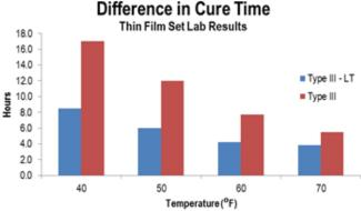
Pro-Poxy Type III DOT LT provides superior performance where it matters: at low temperatures. The colder it gets, the better it out-performs current epoxy systems, while still maintaining enhanced, yet manageable cure times.
