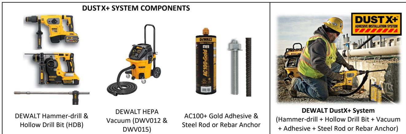
The DustX+ system allows users to drill holes in concrete and masonry and clean the holes during the drilling process at the same time (no extra cleaning steps are necessary with this system). The hollow drill bits are attached to a self-cleaning HEPA vacuum which provide the dust collection during drilling. DEWALT has conducted extensive supplemental laboratory testing on AC100+ Gold adhesive anchors installed in holes drilled and cleaned using the DustX+ system in dry concrete.
