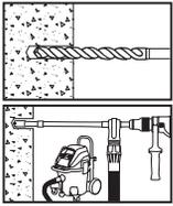
1- Drill a hole into the base material with rotary hammer drill (i.e. percussion drill) and a carbide drill bit to the size and embedment required by the selected steel hardware element (reference installation specifications for threaded rod and reinforcing bar). The tolerances of the carbide drill bits, including hollow bits, must meet ANSI Standard B212.15.
