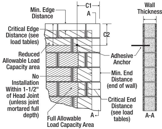
**AC100+ Gold Adhesive Anchors Installed into Top of Grouted Concrete Masonry Wall**
