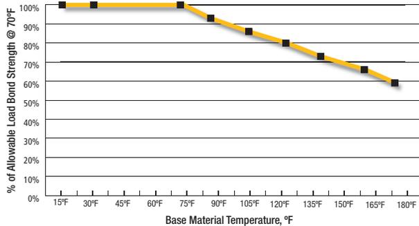
**Load-Temperature Reduction Curve
