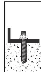
5. Allow the Hammer-Capsule to cure for specified time before loading anchor. Do not disturb, torque or load the anchor once the material has begun to set.
