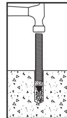
4. Drive the threaded rod or reinforcing bar into the anchor hole through the capsule until it is fully embedded. A 2-pound hammer and eye protection are recommended.
