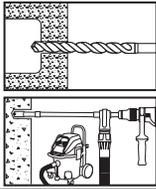
1- Drill a hole into the base material with a rotary drill tool to the size and embedment for the required screen size (see installation specifications for threaded rod in hollow concrete base material with screen tube supplied by DEWALT). Holes drilled in hollow concrete masonry units may be drilled with a rotary hammer-drill. The tolerances of the drill bit used should meet the requirements of ANSI B212.15.
