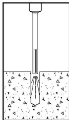
2. Starting from the bottom or back of the anchor hole, remove dust and debris from the hole (e.g. dust extractor) to remove loose particles from drilling, brush the hole with a nylon brush, and again remove any remaining loose particles. Anchor holes may be dry or damp, but should be free of standing water or frost. Vacuuming only is not sufficient. Blow out bulbs generally do not provide enough dust removal for most drilled anchor holes. Holes should be clean and sound
