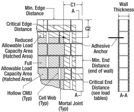
**Direction of Shear Loading in Relation to Edge and End of Masonry Wall**
