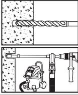
1- Drill a hole into the base material with rotary hammer drill (i.e. percussion drill) and a carbide drill bit to the size and embedment required by the selected steel hardware element (reference installation specifications for threaded rod and reinforcing bar). The tolerances of the carbide drill bits, including hollow bits, must meet ANSI Standard B212.15.
