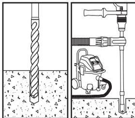
1. Drill a hole using a carbide tipped bit meeting the diameter requirements of ANSI B212.15 to the minimum depth required as shown in the chart.
