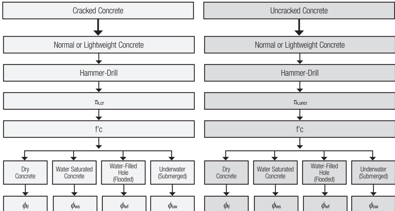
**Bond Strength Design Information for Threaded Rods and Reinforcing Bars<sup>1,2</sup>**
