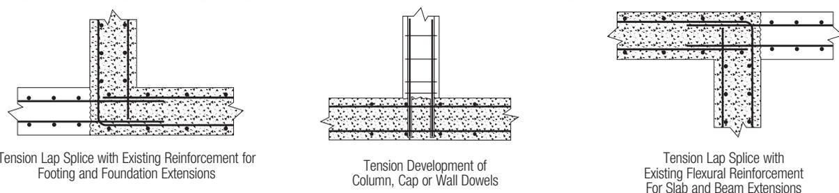
Tension Lap Splice with Existing Reinforcement for Footing and Foundation Extensions
