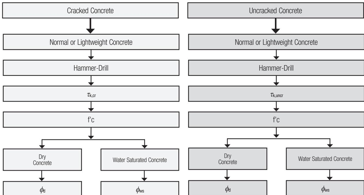
**Concrete Breakout Design Information for Threaded Rod and in Holes Drilled with a Hammer Drill and Carbide Bit<sup>1</sup>**
