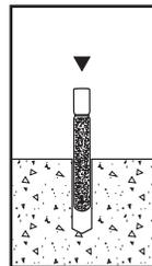
3. Prior to installation check the capsule to be sure it is not damaged and invert several times at 60°F or above to confirm all of the resin is in a liquid state. Insert the capsule into the hole.
