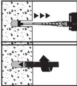
• Piston plugs (see adhesive piston plug table) must be used with and attached to the mixing nozzle and extension tube for horizontal and overhead installations with anchor rod from 5/8" to 1-1/4" diameter and rebar size #5 to #10. Insert piston plug to the back of the drilled hole and inject as described in the method above. During installation the piston plug will be naturally extruded from the drilled hole by the adhesive pressure.
