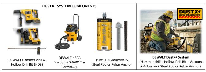
The DustX+ system allows users to drill holes in concrete and clean the holes during the drilling process at the same time (no extra cleaning steps are necessary with this system). The hollow drill bits are attached to a self-cleaning HEPA vacuum which provide the dust collection during drilling. DEWALT has conducted extensive supplemental laboratory testing on Pure110+ adhesive anchors installed in holes drilled and cleaned using the DustX+ system in dry concrete.
