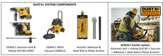
The DustX+ system allows users to drill holes in concrete and clean the holes during the drilling process at the same time (no extra cleaning steps are necessary with this system). The hollow drill bits are attached to a self-cleaning HEPA vacuum which provide the dust collection during drilling. DEWALT has conducted extensive supplemental laboratory testing on Pure50+ adhesive anchors installed in holes drilled and cleaned using the DustX+ system in dry concrete.
