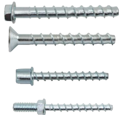
FIGURE 1B—SCREW-BOLT+ (Hex Head and Flat Head Versions) AND HANGERMATE+ (Bottom Pictures – Internally Threaded Head and External Thread Head Rod Hanger Versions)
