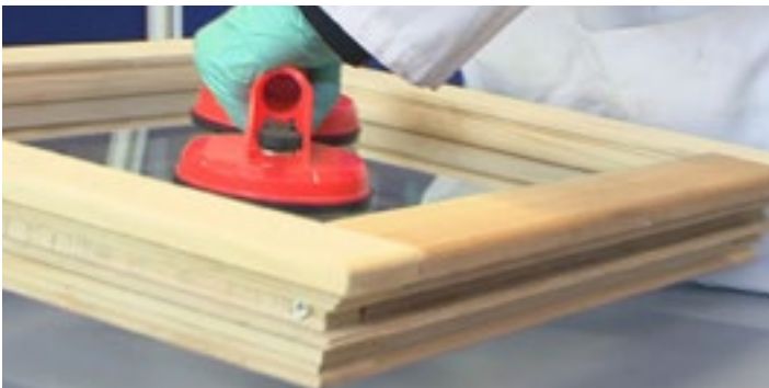
Instant tack enables windows to be moved more quickly after sealant application
