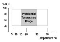
Figure 1: Humidity cure envelope for DOWSIL™ 895 Sealant.
