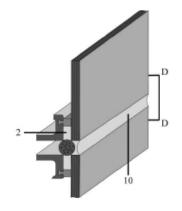
**Figure 3A:** Transom detail. Examples of structural glazing designs: 4-sided design (factory glazed).
