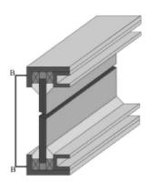
**Figure 2A:** Transom detail. Examples of structural glazing designs: 2-sided design (installed on site).
