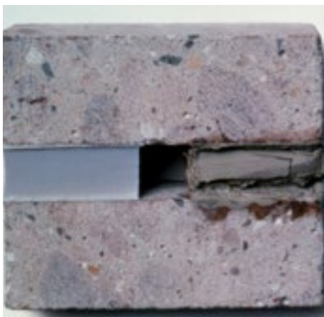
After 100 days (2500 hours) of UV exposure in accelerated weathering and heat stability tests, the urethane sealant deteriorates, while the silicone sealant remains untouched.
