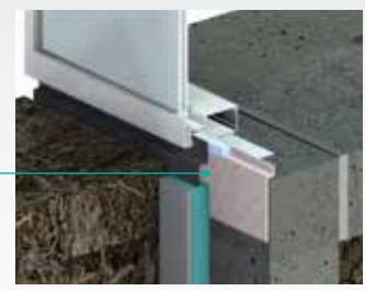
With Dow Corning ® Building Insulation Blanket placed to cover the neck of the curtainwall to the below-grade insulation
