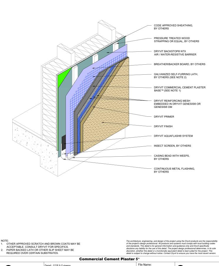
Detail: CCP 5 Cutaway
