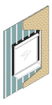
INSTALL WINDOW, SILL AND HEAD FLASHING AND APPLY DRYVIT AQUAFLASH® SYSTEM OVER HEAD FLASHING
