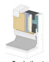
Termination at **Parapet - Solid Substrate**
