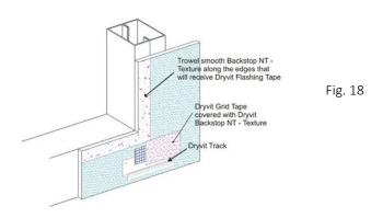
5) The Backstop NT - Texture material should be applied in a uniform, continuous film at the recommended coverage rate. NOTE: Substrates with a surface texture or high porosity will require additional material.
