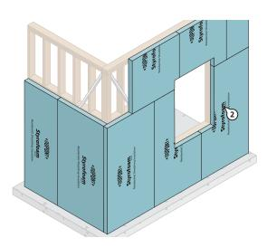
2. Install Styrofoam™ Brand XPS Insulation Products with long edges in contact with one another and all panel edges bearing directly on framing members or blocking. NOTE: 4'x 8', 4'x 9' and 4'x 10' Styrofoam™ Brand XPS Insulation Products may be installed horizontally or vertically. 2' x 8' Styrofoam™ Brand XPS Insulation Products must be installed horizontally.
