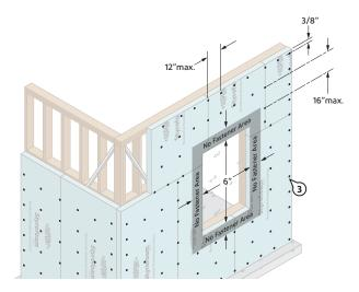
3. Secure **Styrofoam™ Brand XPS Insulation Products** using 3/8″ head (9.5mm) galvanized nails, 1″ crown (25.4mm) galvanized staples, 1″ (25.4mm) head plastic cap nails or equivalent fasteners long enough to penetrate framing a minimum of 3/4″. Fasteners should not be over-driven.
