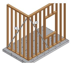
Install a code-acceptable wall bracing (e.g. diagonal metal strapping, let-in wood or wood structural sheathing), see <u>ICC ESR 2142</u> for more information. If wood sheathing is used, it should be covered by **Styrofoam™ Brand XPS Insulation Products** to provide full wall insulation. **NOTE: Styrofoam™ Brand XPS Insulation Products** are not structural panels.
