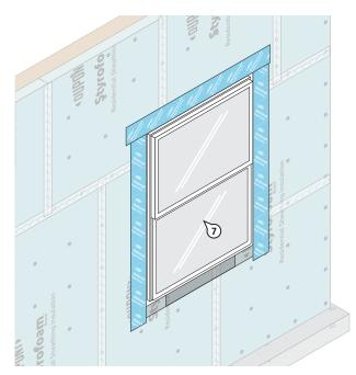
7. Install window per manufacturer's installation instructions. **NOTE**: Fasteners for window installation must be long enough to penetrate at least 1-1/4" (31.8 mm) into the framing.
