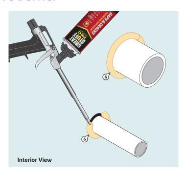
Seal around the interior openings of exterior penetrations with Great Stuff Pro™ Gaps & Cracks Polyurethane Foam Sealant.
