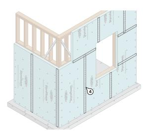
4. Tape all insulation joints (i.e., horizontal and vertical seams) using 2–7/8" (73 mm) wide **DuPont™ Styrofoam™ Brand Tape**.
