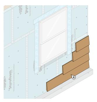
8. Install exterior cladding by fastening through the insulation and into the wood studs in accordance with the cladding manufacturer's instructions.
