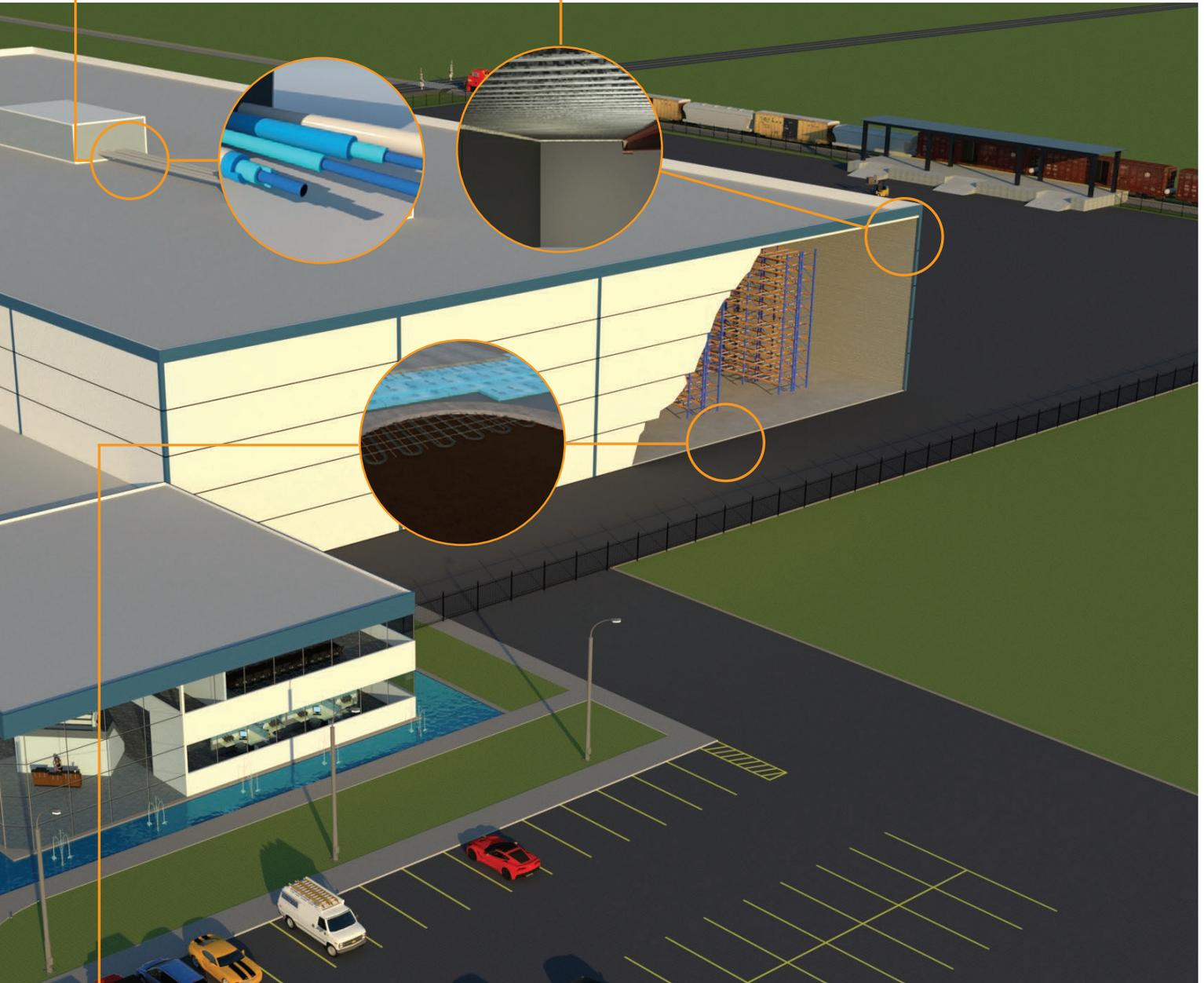
**4 As building heights increase, so does the need for greater compressive strength insulation**
