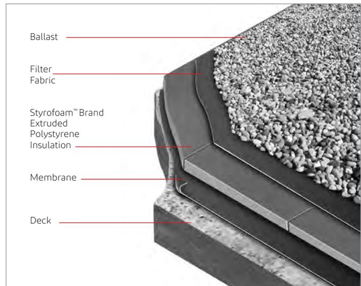
Figure 2: PMR With Membrane Below the Insulation
