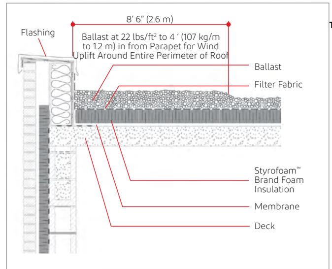
Figure 5: Parapet Detail With Fabric\*\*
