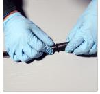
Any exposed end of BEJS must have its exposed vertical face covered with a coat of silicone. Apply silicone to this face.
