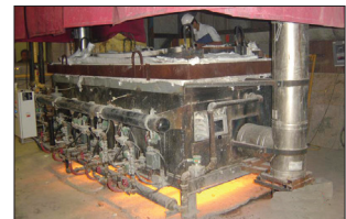
Testing oven below the Emshield DFR2 reaches a maximum temperature of 1850°F (1010°C).
