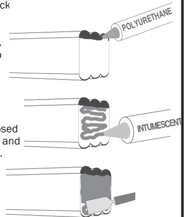
**IMPORTANT:** All sticks of SecuritySeal SSF3 foam MUST have a coating of intumescent on the faces of all joints. This ensures that joints do not compromise the fire barrier.
