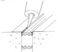
• Where TFR-RWS foam meets at butt joins, tool the excess silicone that squeezes out from the top and between the bellows.
