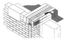
Like the solid-wall closure, the cavity-wall RoofJoint closure, is a factory-fabricated transition piece made from Seismic Colorseal. The difference is an extended, horizontal setback portion of coated foam to bridge the cavity from facade to structural backup wall. The sides of the "bridge" are additionally seated with silicone to seal them against
