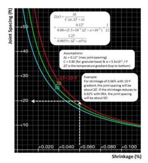
This graph shows typical recommended joint spacing criteria (Darter and Barenberg, 1977) and has been used in FHWA reports and multiple publications.
