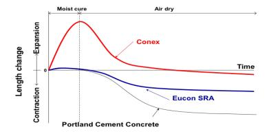
The graph on the left shows the shrinkage typically experienced in reference Portland cement based concrete and concrete utilizing *Shrinkage Reducing admixtures* and *Shrinkage Compensating materials*.
