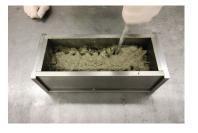
Fill in 2 equal layers and properly consolidate each by rodding 45 times per layer and lightly tapping the outside of the mold 10-15 times with the mallet. If using fiber reinforced concrete, use external vibration only.
