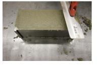
After consolidating the beam, strike off excess material with a straight edge and clean the excess paste from the mold.
