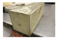
IMMEDIATELY after demolding, an initial comparator reading must be made. This step is critical, as this measurement will be used as the initial reading for future length change calculations. Due to the nature of CONEX and its expansive properties, this modification is necessary because 90% of expansion occurs in the first 24 hours.
