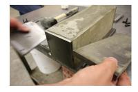
At 12 hours carefully remove the specimen from the mold. Care must be taken not to disturb the pins and this area should remain free from any cracks or damage. The pins should be set firmly in place of the concrete on each end.
