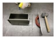
Before inserting the gauge pins into the mold, lightly spray the mold with a form release to ensure the specimen does not become damaged while demolding.
