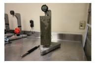
Finally, after the 7 day wet cure, remove the specimen from the lime water bath and place in a temperature and humidity controlled room at  $50 \pm 4\%$  RH and a temperature of  $73 \pm 3^{\circ}$  F. Make subsequent air storage readings at 7, 14, 21 and 28 days. Continue this process if additional measurements past 28 days are needed.
