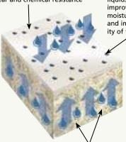
Penetrating sealers are breathable and allow moisture in cured concrete to escape. This reduces the risk of rebar corrosion
