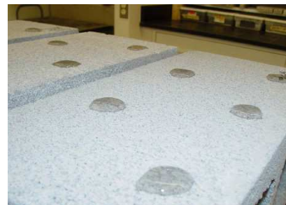
WATER BEAD TEST
