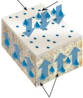
Penetrating sealers are breathable and allow moisture in cured concrete to escape. This reduces the risk of rebar corrosion
