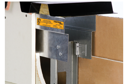
Posi Klips used with Fire Trak Deflection Track and Firestopping System
