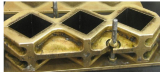
A. 2" x 2" Brass cube mold
