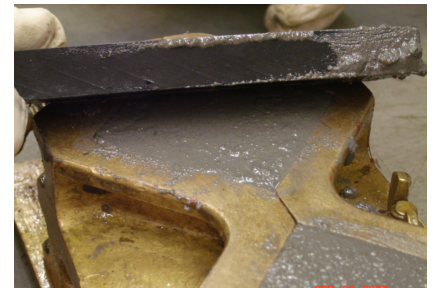
D.5. Screed off excess grout.
