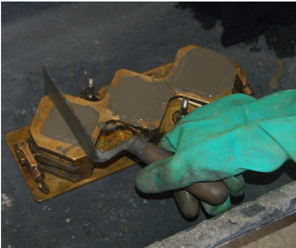
Clean off excess material from the top of the mold.
