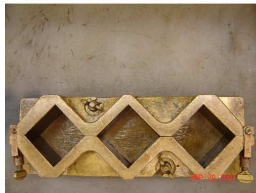
2" x 2" brass cube mold with cover plate
