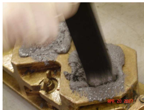
Fill molds halfway with epoxy grout then tamp or rod to remove entrapped air.
