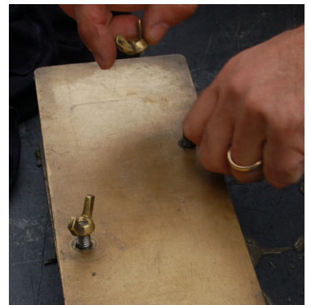
D.6. Place cover plate on mold and tighten with screws or clamps.
