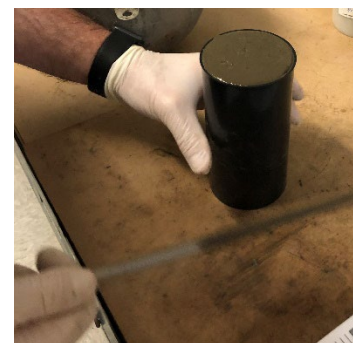
C.1.f. Tap cylinder 10-15x to release air
