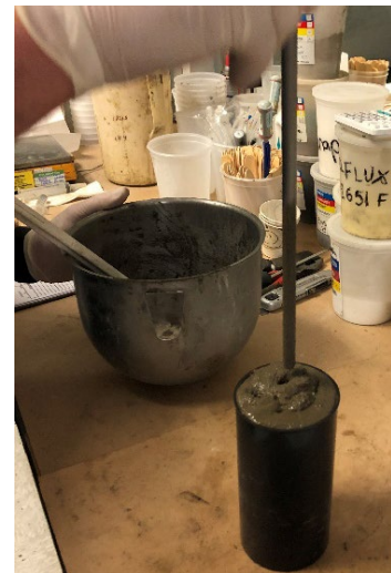
C.1.b. Rod mortar 25 times per lift
