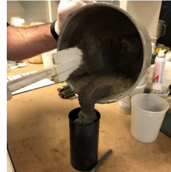
C.1.a. Fill cylinder halfway with mortar
