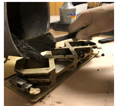
C.2.a. Fill cube mold halfway with mortar
