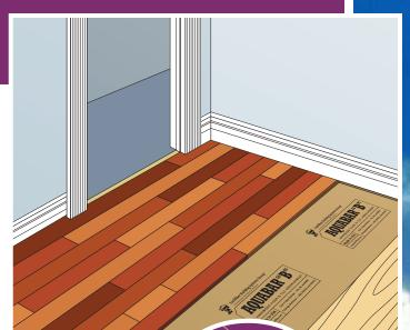
Aquabar "B" hardwood floor and tile underlayment is an extremely effective moisture vapor retarder for use in a variety of interior construction applications. Consisting of two layers of kraft paper laminated with asphalt, Aquabar "B" is a nono-reinforced 30/30/30 duplex type Grade "B" paper.
