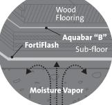
FortiFlash protects floating laminate and engineered floors installed over concrete.
