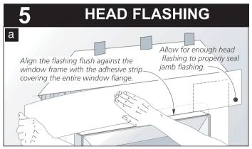
Wipe the head flange, jamb flashing, weather-resistive barrier, and sheathing with a clean rag. Cut a piece of flashing long enough to ensure that the head flashing extends a minimum 1" beyond the jamb flashing. Install the head flashing by pressing firmly in place in one direction to prevent voids.
