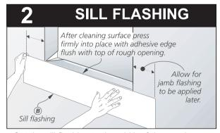
Cut the sill flashing to the width of the rough opening plus twice the flashing width. Wipe the surface of the weather-resistive barrier with a clean rag to ensure proper adhesion. Remove the release paper and press the sill flashing in place so that the edge of the flashing's adhesive is level with the top edge of the rough opening.
