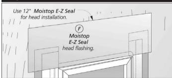
Cut a strip of **Moistop E-Z Seal** for the head **(F)** of the window extending beyond the jamb flashing already in place. Place the **Moistop E-Z Seal** on top of the flange **(D)** of the window with the adhesive strip overlaying the flange and seal by applying pressure along the strip. If desired, staples or sealant may be used to secure the top corners of the head flashing in place.
