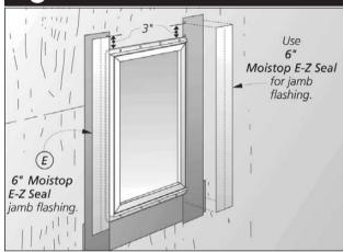
Using a sharp knife, cut the desired length of **Moistop E-Z Seal** for the jamb **(E)** of the window, extending beyond the flange (3" minimum top and bottom). Place the **Moistop E-Z Seal** on top of the flange **(D)** and seal by applying pressure along the strip. Repeat for the other jamb.
