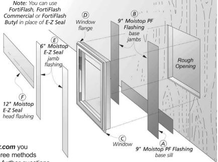
**Note**: You can use **Moistop neXT** in place of **Moistop PF** in base flashing applications.
