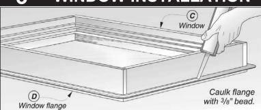
Before installing the window (C), apply a continuous <sup>3</sup>/<sub>8</sub>" bead of **Moistop Sealant** to the perimeter of the rough opening or to the backside of the mounting flange (D) of the window. Install the window according to the window manufacturer's instructions.
