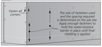
Under normal conditions, attaching the water-resistive barrier with a quality exterior grade staple is acceptable. A higher grade of galvanized fastener, or large headed galvanized nail may be required in certain settings or weather conditions.
