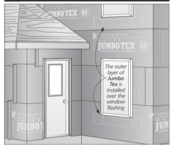
An outer layer of **Jumbo Tex** is now installed over the first water-resistive barrier layer in weather-board fashion, following the same requirements for overlaps and fasteners. However, this layer is not integrated with the window flashing, but is instead installed over the integrated flashing and first water-resistive barrier.
