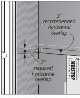
Any succeeding course should be placed horizontally over the lower course in a weather-board fashion with a minimum horizontal overlap of 2" (3" is recommended)
