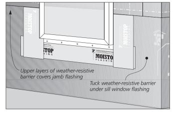
When a course of the water-resistive barrier first crosses the path of any window, it needs to be properly integrated with the window sill and jamb flashing for quality moisture management. To do this, tuck water-resistive barrier under the sill and jamb flashing as shown above. The courses above this point can butt into the window jamb.
