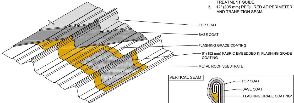
\*Trapezoidal seams may forgo flashing grade treatment with approval via a Field Services pre-job inspection.
