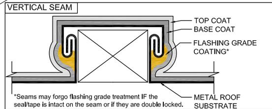
\*Seams may forgo flashing grade treatment IF the seal/tape is intact on the seam or if they are double locked.
