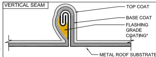
\*Seams may forgo flashing grade treatment IF the seal/tape is intact on the seam or if they are double locked.
