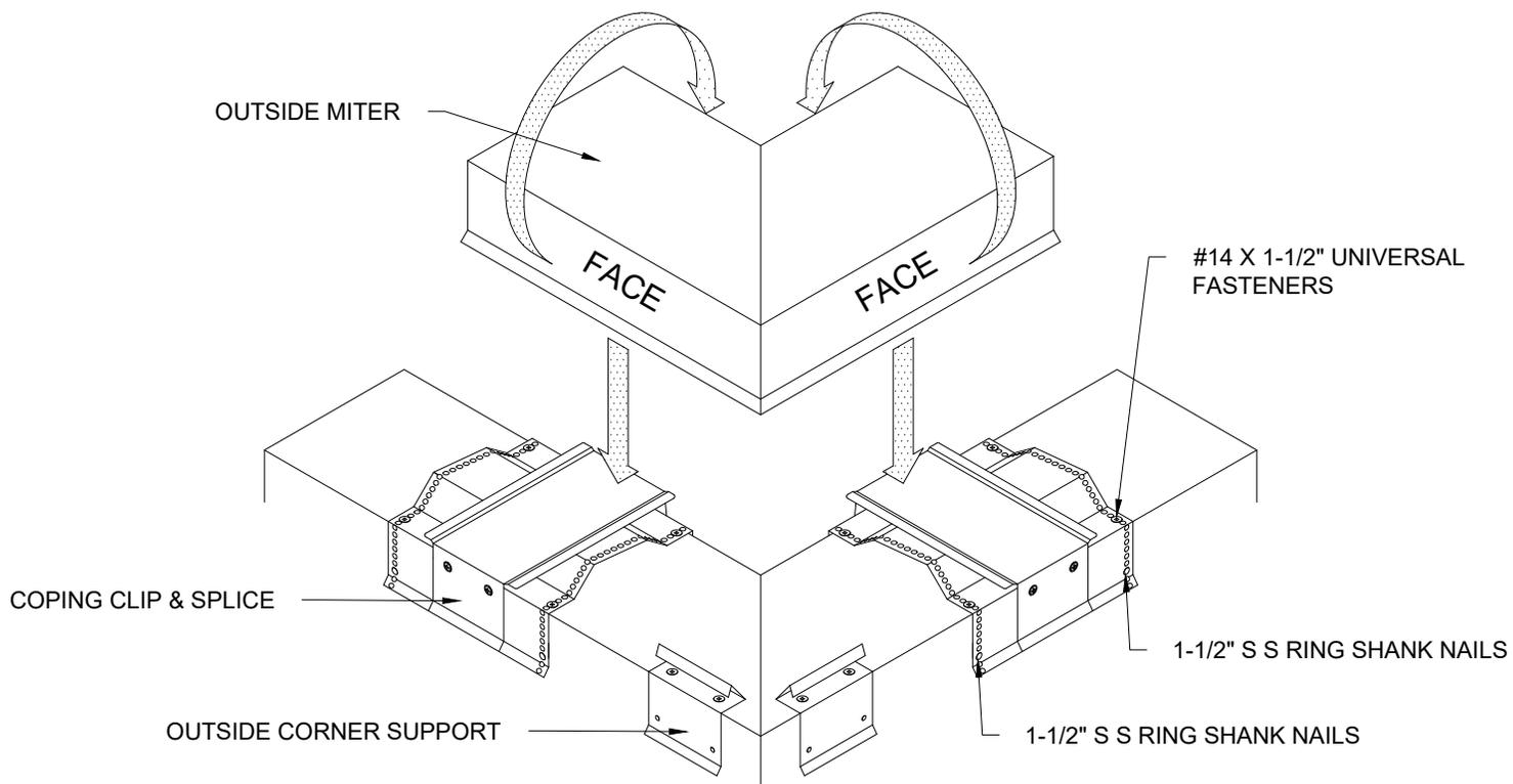
**STEP 5: PLACE CLIPS AT END LOCATIONS SHOWN BELOW AND LOCATE END CAPS/END TERMS AND HOOK ON FRONT OF CLIP, ROTATE BACKWARD AND PRESS DOWNWARD TO ENGAGE ONTO CLIP. \*SECURE ENDCAP TO CLIP USING POP-RIVET OR SCREW (BY INSTALLER) TO PREVENT LATERAL MOVEMENT.**
