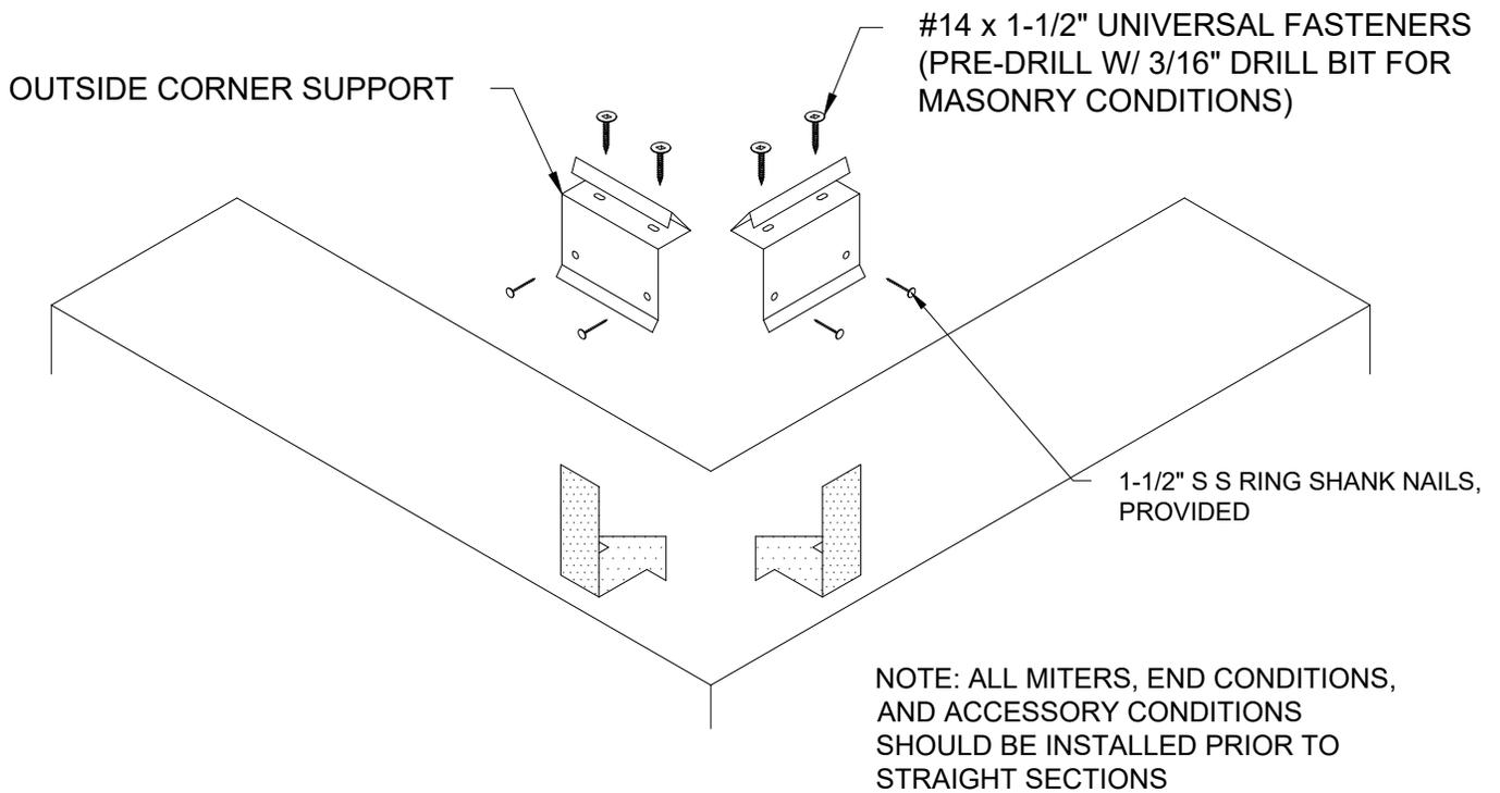
**STEP 2: ALIGN CENTER OF EACH CLIP FROM THE CORNER SUCH THAT THE MITER LEG SITS HALF-WAY OVER EACH CLIP AS SEEN IN STEPS 3 & 4 (PAGE 4)**
