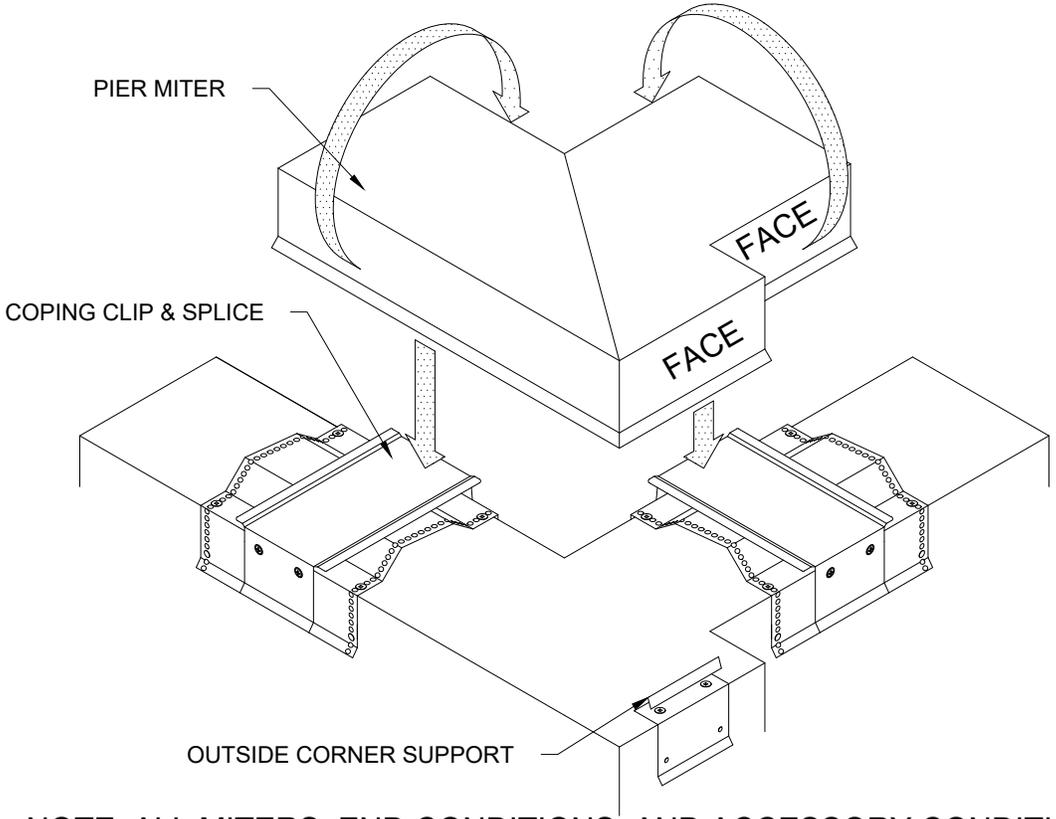
NOTE: ALL MITERS, END CONDITIONS, AND ACCESSORY CONDITIONS SHOULD BE INSTALLED PRIOR TO STRAIGHT SECTIONS
