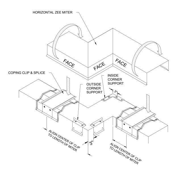
NOTE: ALL MITERS, END CONDITIONS, AND ACCESSORY CONDITIONS SHOULD BE INSTALLED PRIOR TO STRAIGHT SECTIONS
