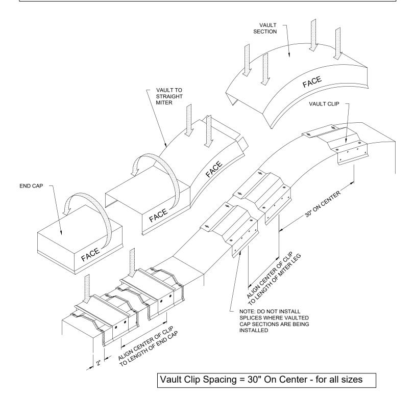
NOTE: ALL MITERS, END CONDITIONS, AND ACCESSORY CONDITIONS SHOULD BE INSTALLED PRIOR TO STRAIGHT SECTIONS
