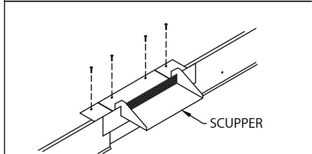
4. INSTALL SCUPPER WITH PROVIDED FASTENERS. ROOF MEMBRANE IS INSTALLED UNDER SCUPPER. SET SCUPPER FLANGE IN A CONTINUOUS BEAD OF NON-CURING SEALANT (BY OTHERS).
