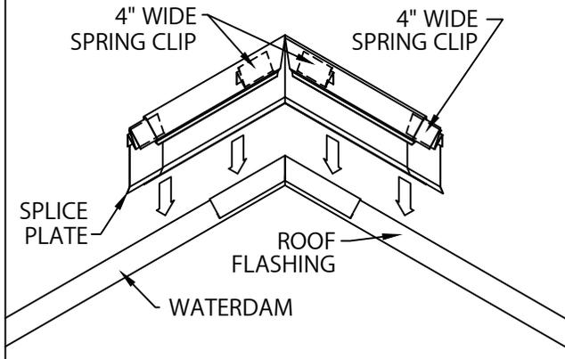
10. INSTALL MITER COVERS FIRST. INSERT ONE SPLICE PLATE AND ONE 4" WIDE SPRING CLIP INTO EACH END OF MITER COVER, HALF EXPOSED (SEE DETAIL BELOW FOR PROPER SPRING INSTALLATION). PLACE TWO 4" WIDE SPRING CLIPS INTO CORNERS OF MITER AS SHOWN. INSTALL MITER COVERS BY PUSHING DOWNWARD UNTIL COVER IS ENGAGED ALONG ENTIRE MITER.
