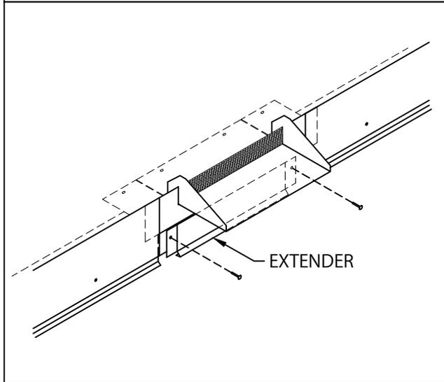
6. CENTER EXTENDER BELOW SCUPPER AND FASTEN THROUGH PRE-SLOTTED HOLES WITH PROVIDED FASTENERS AS SHOWN.
