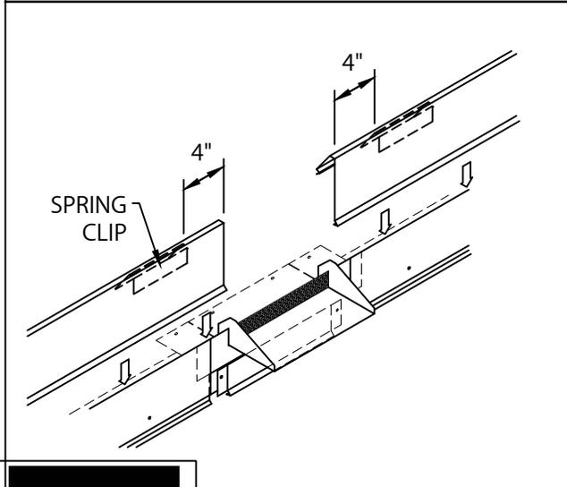
7. PLACE SPRING CLIPS 4" FROM END OF FASCIA COVER. INSTALL COVER BY PUSHING DOWNWARD UNTIL FASCIA COVER IS ENGAGED TO WATERDAM. FASCIA COVER SHOULD FIT TIGHT AGAINST SIDES OF SCUPPER.
