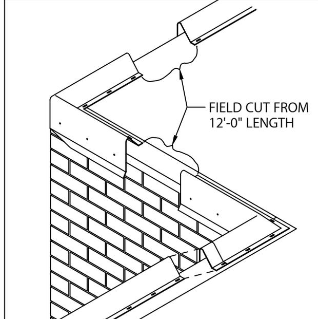
2. LOCATE AND INSTALL MITERS, FASTEN THROUGH PRE-SLOTTED FASTENING HOLES ON TOP OF NAILER AND OUTSIDE FACE. DETERMINE AND IDENTIFY LOCATION OF SCUPPERS. DO NOT INSTALL SCUPPERS AT THIS TIME. LEAVE GAP OF 14 1/2" INCHES FOR SCUPPER LOCATIONS. THEN INSTALL THE 12'-0" SECTIONS OF WATERDAM FROM RIGHT TO LEFT (AS SEEN FROM ROOF TOP) BY FASTEN THROUGH SLOTTED HOLES PROVIDED PER JOB REQUIREMENTS. FIELD CUT SECTIONS AS NECESSARY. LAP WATERDAM JOINTS 1".
