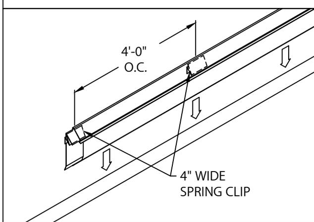
11. INSTALL 12'-0" FASCIA COVER SECTIONS. INSERT ONE SPLICE PLATE AND ONE 4" WIDE SPRING CLIP UNDER FAR END OF FASCIA COVER, HALF EXPOSED. PLACE 4" WIDE SPRING CLIPS INTO COVER AT 4'-0" O.C. INSTALL COVER BY PUSHING DOWNWARD UNTIL FASCIA COVER IS ENGAGED TO WATERDAM ALONG ENTIRE LENGTH. CONTINUE TO INSTALL FASCIA COVERS, LEAVING A 3/8" SPACE BETWEEN COVERS. FIELD CUT WHERE NECESSARY USING FINE TOOTH HACKSAW.
