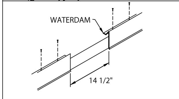
3. DETERMINE LOCATION OF SCUPPER AND SPACE WATERDAM 14 1/2" APART AS SHOWN. FASTEN WATERDAM FLANGE 6" O.C. WITH PROVIDED FASTENERS.
