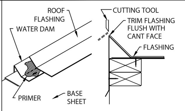
8. USE APPROPRIATE TYPE AND WIDTH OF ROOF MEMBRANE FLASHING. METAL ASPHALT PRIMER IS NECESSARY TO FLASH UP THE CANT OF THE WATERDAM. TRIM OVERHANGING FLASHING FLUSH WITH FACE OF CANT. CONSULT ROOFING MANUFACTURER FOR PROPER MATERIALS PROCEDURE FOR STRIPPING IN WATERDAM WITH FLASHING.
