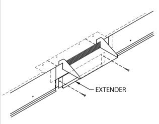
6. CENTER EXTENDER BELOW SCUPPER AND FASTEN THROUGH PRE-SLOTTED HOLES WITH PROVIDED FASTENERS AS SHOWN.
