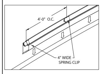
2. INSTALL 12'-0" FASCIA COVER SECTIONS. INSERT ONE SPLICE PLATE AND ONE 4" WIDE SPRING CLIP UNDER FAR END OF FASCIA COVER, HALF EXPOSED. PLACE 4" WIDE SPRING CLIPS INTO COVER AT 4'-0" O.C. INSTALL COVER BY PUSHING DOWNWARD UNTIL FASCIA COVER IS ENGAGED TO WATERDAM ALONG ENTIRE LENGTH. CONTINUE TO INSTALL FASCIA COVERS, LEAVING A 3/8" SPACE BETWEEN COVERS. FIELD CUT WHERE NECESSARY USING FINE TOOTH HACKSAW.
