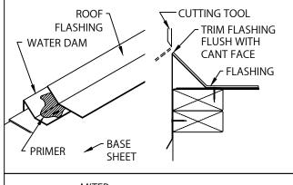
8. USE APPROPRIATE TYPE AND WIDTH OF ROOF MEMBRANE FLASHING. METAL ASPHALT PRIMER IS NECESSARY TO FLASH UP THE CANT OF THE WATERDAM. TRIM OVERHANGING FLASHING FLUSH WITH FACE OF CANT. CONSULT ROOFING MANUFACTURER FOR PROPER MATERIALS PROCEDURE FOR STRIPPING IN WATERDAM WITH FLASHING.
