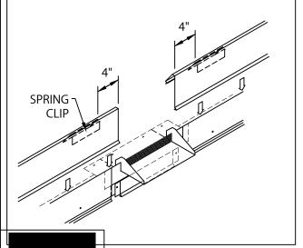
7. PLACE SPRING CLIPS 4" FROM END OF FASCIA COVER. INSTALL COVER BY PUSHING DOWNWARD UNTIL FASCIA COVER IS ENGAGED TO WATERDAM. FASCIA COVER SHOULD FIT TIGHT AGAINST SIDES OF SCUPPER.
