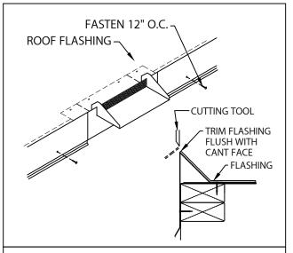
5. POSITION ROOF FLASHING UP FASCIA AND SCUPPER WATERDAM. TRIM FLASHING FLUSH WITH CANT AS SHOWN. FASTEN WATERDAM 12" O.C. THROUGH ALL RAISED FASTENING HOLES ON OUTSIDE FACE USING PROVIDED FASTENERS.
