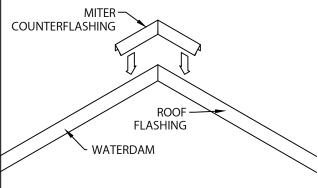
9. PLACE MITER COUNTERFLASHING ON CORNER.
