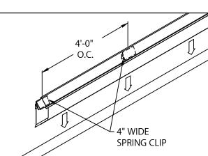
11. INSTALL 12'-0" FASCIA COVER SECTIONS. INSERT ONE SPLICE PLATE AND ONE 4" WIDE SPRING CLIP UNDER FAR END OF FASCIA COVER, HALF EXPOSED. PLACE 4" WIDE SPRING CLIPS INTO COVER AT 4'-0" O.C. INSTALL COVER BY PUSHING DOWNWARD UNTIL FASCIA COVER IS ENGAGED TO WATERDAM ALONG ENTIRE LENGTH. CONTINUE TO INSTALL FASCIA COVERS, LEAVING A 3/8" SPACE BETWEEN COVERS. FIELD CUT WHERE NECESSARY USING FINE TOOTH HACKSAW.
