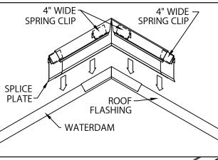
10. INSTALL MITER COVERS FIRST. INSERT ONE SPLICE PLATE AND ONE 4" WIDE SPRING CLIP INTO EACH END OF MITER COVER, HALF EXPOSED (SEE DETAIL BELOW FOR PROPER SPRING INSTALLATION). PLACE TWO 4" WIDE SPRING CLIPS INTO CORNERS OF MITER AS SHOWN. INSTALL MITER COVERS BY PUSHING DOWNWARD UNTIL COVER IS ENGAGED ALONG ENTIRE MITER.
