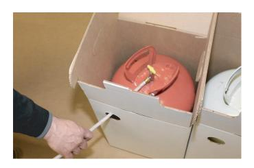
**STEP 4.** Attach swivel fitting on red striped hose, finger tight, to the valve outlet on top of the red cylinder.
