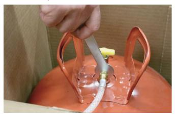
**STEP 7.** Fully open the valves on the canisters using both hands, if needed. Do not use a tool to try to open a valve that is difficult to open. Point applicator into bucket or garbage can. Hold trigger lock up and engage trigger to spray into receptacle. Ensure even flow from both sides. If flow is not even, check that both canister valves are fully open and re-spray.
