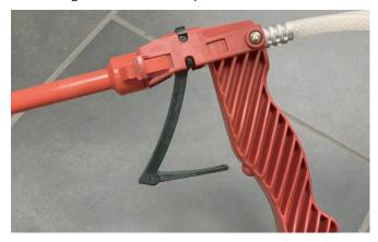
**STEP 9.** It is recommended to verify the canisters are properly reacting and curing before using. Spray onto scrap piece of substrate (iso, deck or coverboard) and monitor the reaction.
