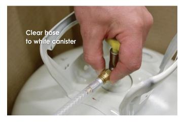
**STEP 6.** Tighten both fittings with the 9/16-in. wrench (provided) by turning an additional 1/6 turn until firmly attached. DO NOT OVER- TIGHTEN! Close lid of each box to protect from sun, wind and dirt.
