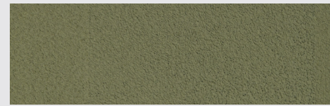
SR Limestone (SRI = 55) Reflectance: .47 Emittance: .87
