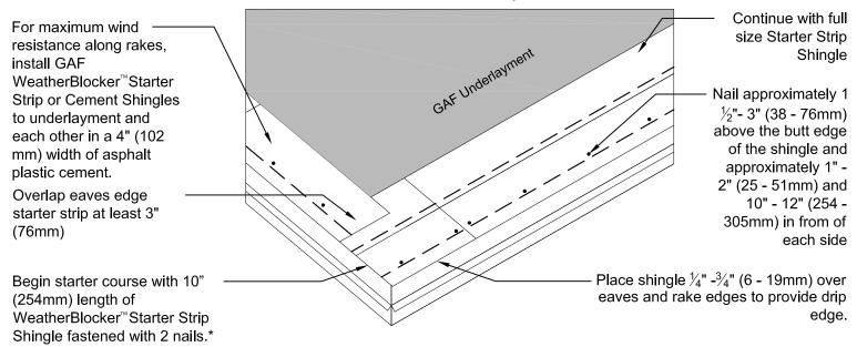
Note: For all applications, the butt joints of the Weather Blocker™ Starter Shingles must be offset from the butt joints of the first course of shingles by 4" or more. For long eaves, a 10" (254 mm) piece of Weather Blocker™ Starter may need to be installed periodically to adjust the offset. The frequency of this adjustment will depend on the length of the shingles being installed.
