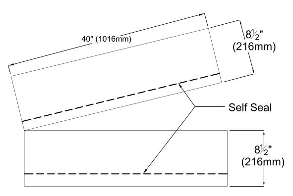
Seperate WeatherBlocker<sup>™</sup>Starter Strip Shingle horizontally along perforation when used at eaves with shingles with exposures less than 6" (152mm)
